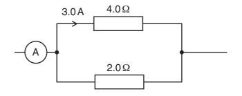
The current in the  $4.0\Omega$  resistor is 3.0 A.
